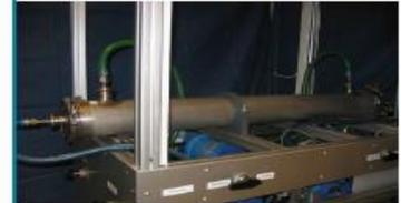
Experimental set-up for membrane development for harnessing salinity gradient energy Osmotic Power
